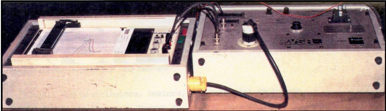
**VSR-752 Control Console and Plotter. Plotter has completed VSR Treatment Chart #1**
